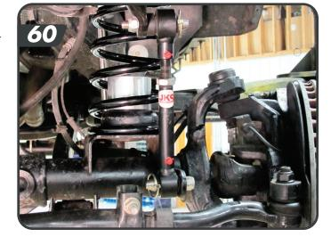
The front brake line brackets have a tab that inserts into the OE frame slot with the bracket towards the rear of the slot. Attach the drop brackets to the brake line so the brake line tab fits into the drop bracket slot using the provided 1/4" hardware. [61]
