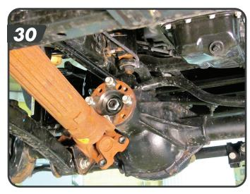
Disconnect the steering drag link from the pitman arm to ensure it doesn't bind when installing the new coil springs. Remove the tie rod end nut and dislodge the tie rod end from the pitman arm. Save nut. [31]
