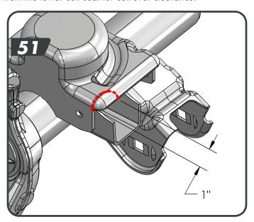
bc. Remove the control arm nut. Place the control arm mount cam plate in between the cam stops on the axle mount. Note: The axle bracket kit is not compactible with an off center control arm bolt from an alignment bolt or cam washer. Longer or adjustable replacement control arms will be required to adjust the caster on the vehicle.
