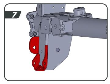
b. Measure 1.5" down from the center of the lower control arm mounting hole and make a cut perpindicular to the rear face of the mount [8].
