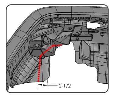
b. Fasten the inner fenders to the body with the original hardware.
