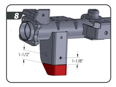
Drill out the the 2 factory holes on the rear face of the mount using a  $\frac{1}{2}$ " drill bit [9].
