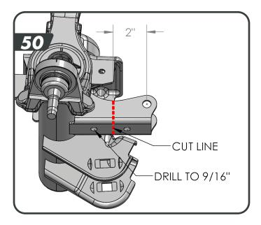
ba. Drill out the remaining hole in the shock mount to 9/16"
